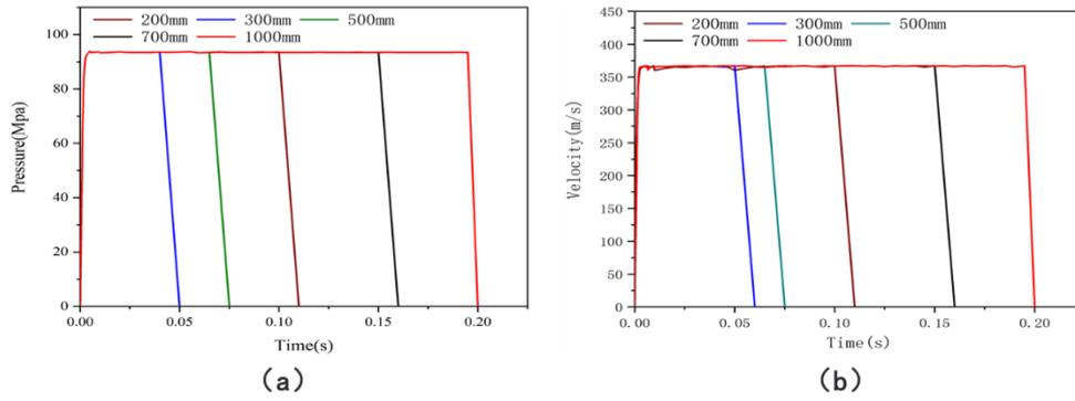
**Figure 6 In different plunger stroke intensifier output pressure characteristic curve**
