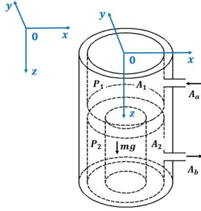
**Figure 3 plunger movement model of the intensifier**
