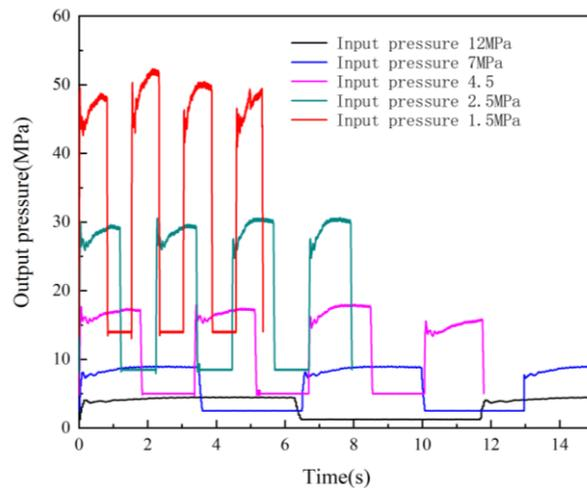
Figure.11 Laboratory test curve of intensifier output characteristics
