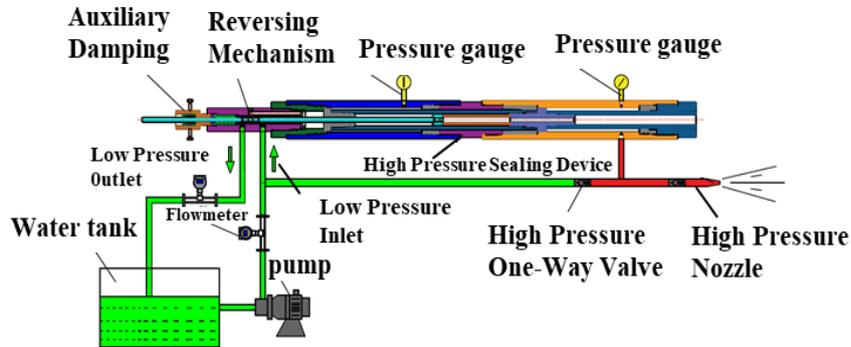
Figure 9 Schematic diagram of intensifier laboratory test
