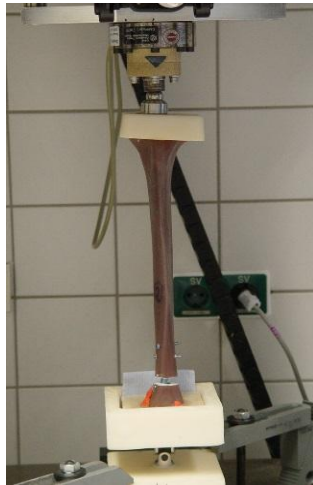
Figure 2. Test set-up for axial testing.
