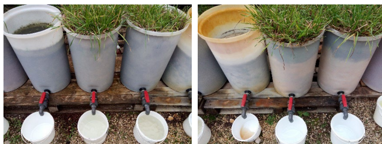
Fig 1 Lysimeters of TF mine tailings (left: control #9, treated with MBR #10, treated with limestone #11) and of T1 mine tailings (right: control #12, treated with MBR and limestone #13, treated with limestone #14). The orange color on the walls of the lysimeter #12 and in the bucket is iron oxide
