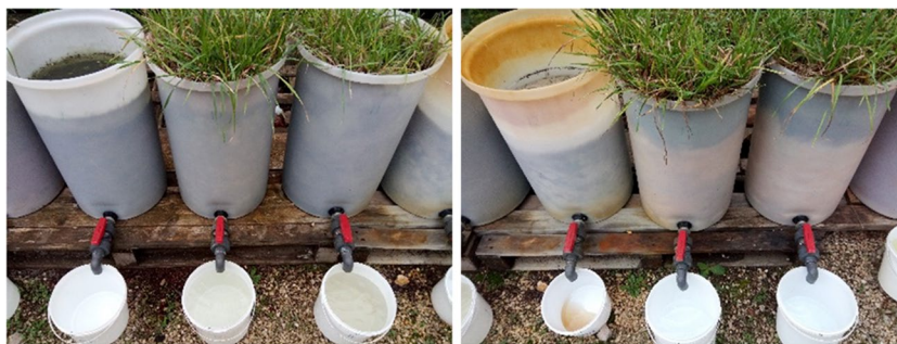
Fig. 1 Lysimeters of TF mine tailings (left picture, from left to right: control #9, treated with MBR #10, treated with limestone #11) and of T1 mine tailings (right picture, from left to right: control #12,
