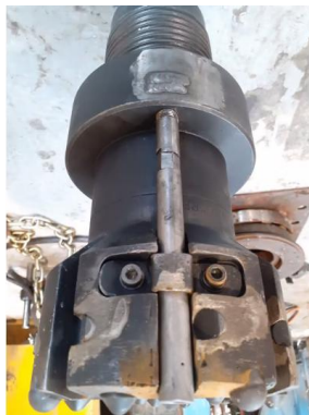
Figure 12: Modified hammer drill bit with HPWJ nozzle
