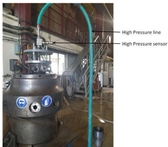
Figure 5: The high pressure impact cell modified to accommodate the high pressure water jetting experiments.
