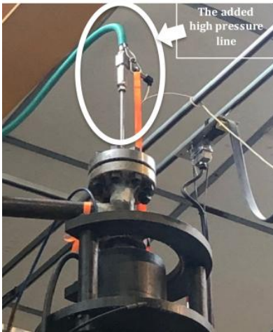
Figure 10: Modified swivel to allow High Pressure Water line on rotating drillstring
