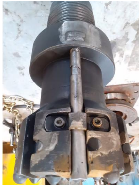
Figure 12: Modified hammer drill bit with HPWJ nozzle
