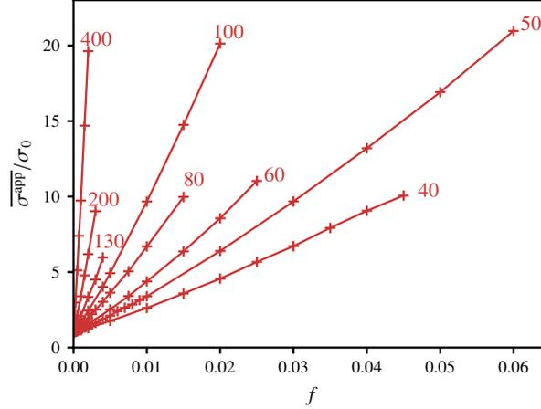
Figure 7: Mean apparent conductivities along volume fraction with EIM, for different aspect ratios (contrast of  $10^6$ , and  $D = 4L$ ). The aspect ratios are precised at the end of each curve.
