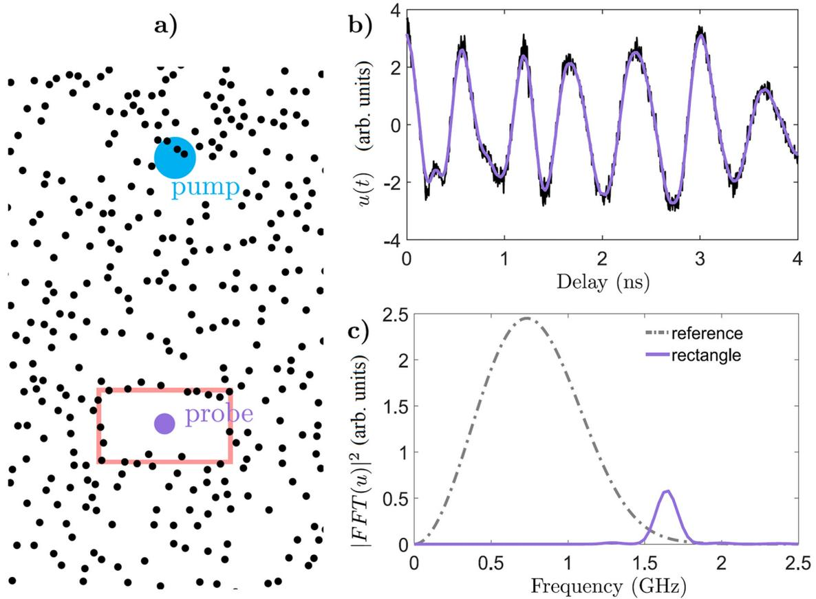
**FIG. 4.** (a) Configuration of the measurement: the pump (blue) and the probe (purple) are separated by  $10\ \mu\text{m}$ . The red rectangle highlights the cavity most studied in this work. (b) Out-of-plane displacement  $u$  measured over 4 ns, directly inside the cavity 0.5 ns after the passage of the elastic wavefront. (c) Spectral content of the vibrations measured inside the cavity.
