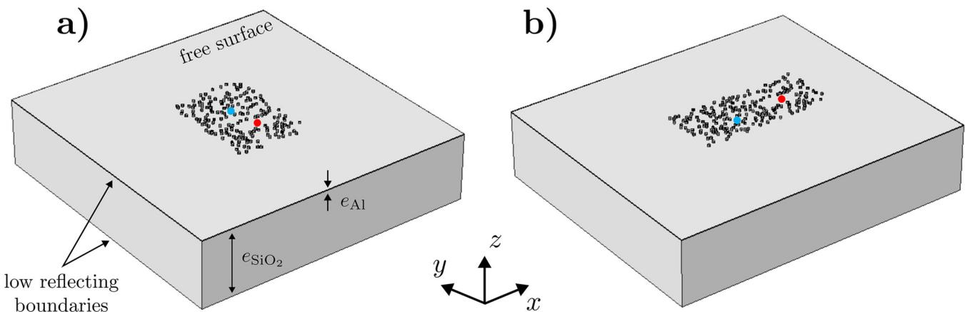
**FIG. 9.** (a), (b) Depiction of the extended geometry model for the perpendicular and parallel main dimensions of the rectangle, respectively. A low reflection boundary condition is applied on the side and the bottom of the geometry while the upper surface is set free. The dimensions of the sample are the same as those in Fig. 7. Blue and red spots highlight the source load and the probe registering the temporal signal.
