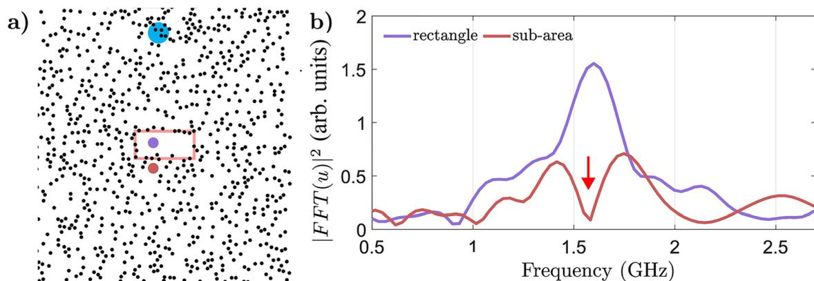
**FIG. 5.** (a) Experimental configuration of the measurement, where the distance between the pump and the probe inside the rectangular cavity is fixed at  $10\ \mu\text{m}$ . (b) Comparison of the Fourier transform between the signal measured inside the rectangular cavity (purple) and in the sub-area (red), 0.5 ns after the passage of the wavefront. The color of the curves corresponds to the color of the probes. The red arrow indicates the resonant frequency of the rectangular cavity.
