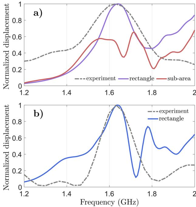
**FIG. 8.** Normalized displacements of the scattered field  $\|w_s\|$  vs frequency for (a) perpendicular and (b) parallel configurations. The spectrum for the rectangle is the average between the three probes in the corresponding area while the spectrum registered in the sub-area is for only one probe, as highlighted by the red spots in Figs. 7(a) and 7(b). These are overlaid by the experimental results, represented as dashed-dotted lines.
