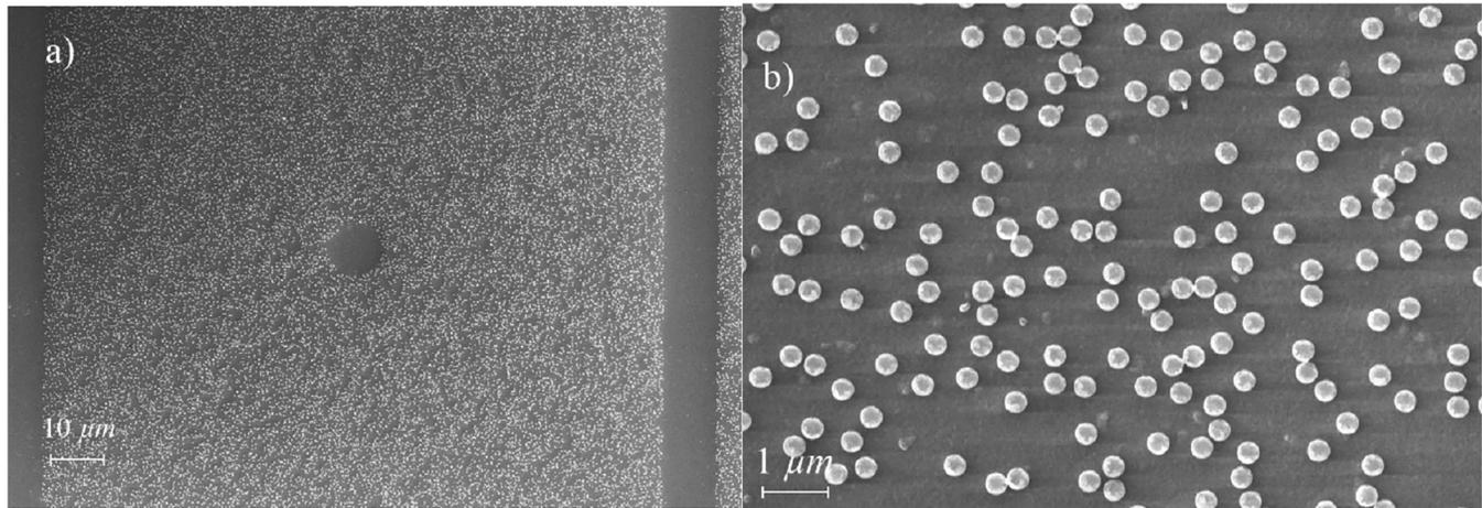
**FIG. 1.** SEM images of (a) wide field and (b) zoom of a random distribution of Al scatterers. The pillars of diameter  $\varphi \sim 320$  nm and height  $h \sim 200$  nm are distributed on an area of  $120 \times 120 \mu\text{m}^2$  and are fabricated on an Al layer of thickness  $e \sim 100$  nm itself deposited on a  $\text{SiO}_2$  substrate.
