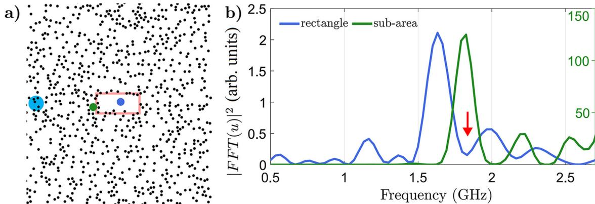
**FIG. 6.** (a) Configuration of the pump-probe measurements such that the distance between the pump and the probe is set at  $10\ \mu\text{m}$ . (b) Comparison of the Fourier transform between the signal measured inside the rectangular cavity (blue) and the in sub-area (green)  $0.5\ \text{ns}$  after the passage of the wave. The colors of the curves correspond to those of the probes. The red arrows indicate the resonant frequencies of the sub-area before the rectangular cavity.
