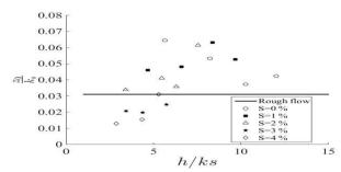
Figure.12. Hydraulic roughness as a function of the relative water depth.
