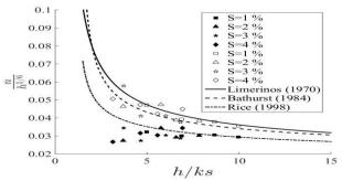
Figure.9. Friction coefficients compared to formula from literature. Open signs correspond to calculus with  $h_{ref} = h$ and full signs to calculus with  $h_{ref} = h - k_s$
