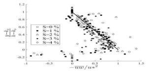
Figure.13. Vertical distribution of Reynolds shear stress
