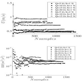
Figure.7. Statistical convergence of velocity (Top) and Reynolds stress (Bottom) at the center of the picture at 2 cm from the bottom.
