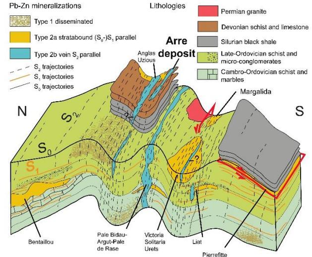
**Figure 1:** Schematic 3D sketch presenting the three main types of mineralization which are typically observed in the studied area and related to each studied deposit. Type 2b vein mineralizations appear in intensely  $S_2$  deformed domains. Location of Arre deposit is noted (modified from Cugerone et al., 2018b)
