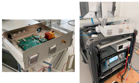
Fig. 2. Transmitter front-end (left) and rack (right)
