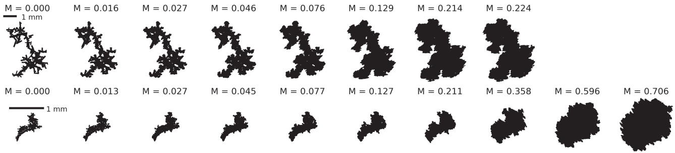
FIGURE 1 Growth of two example aggregates by riming when exposed to an effective liquid water path (ELWP) of 2.0 \text{ kg} \cdot \text{m}^{-2} . Top: aggregate of 300 needles with mean monomer crystal sizes of 200 \mu\text{m} . Bottom: aggregate of 30 dendrites with mean monomer crystal sizes of 100 \mu\text{m} . The rimed aggregates consist of cubic volume elements with 20\text{-}\mu\text{m} width; the scale, shown in the first panel, is the same for images of each row. The normalized rime mass M at the different stages is included above each image. The larger needle aggregate does not reach higher M values than 0.224 with the chosen ELWP.
