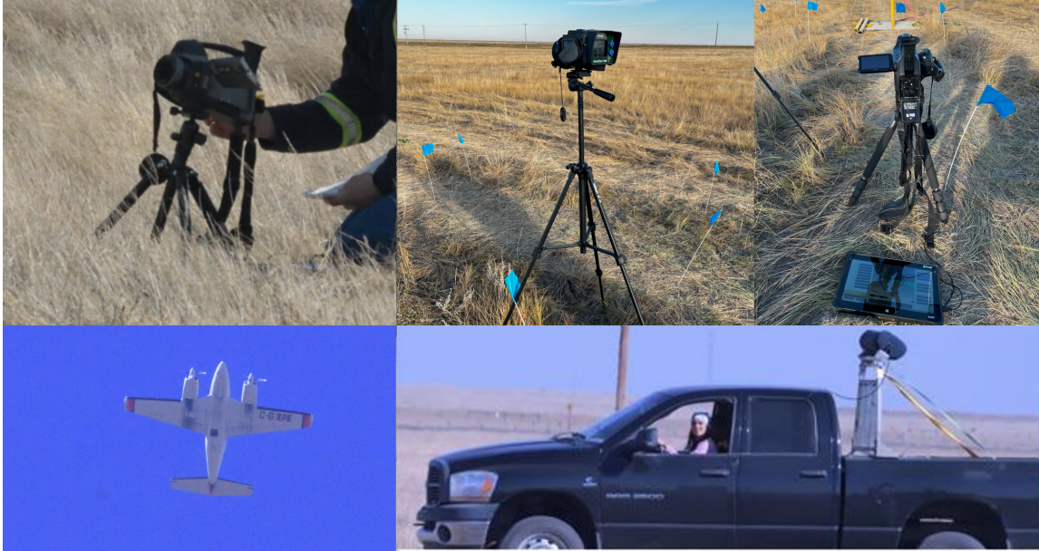
Figure 1: Technologies studied in the field trials. Top row, left to right: QOGI A, QOGI B, QOGI C. Bottom row, left to right: airborne NIR HSI, truck-based TDLAS.
