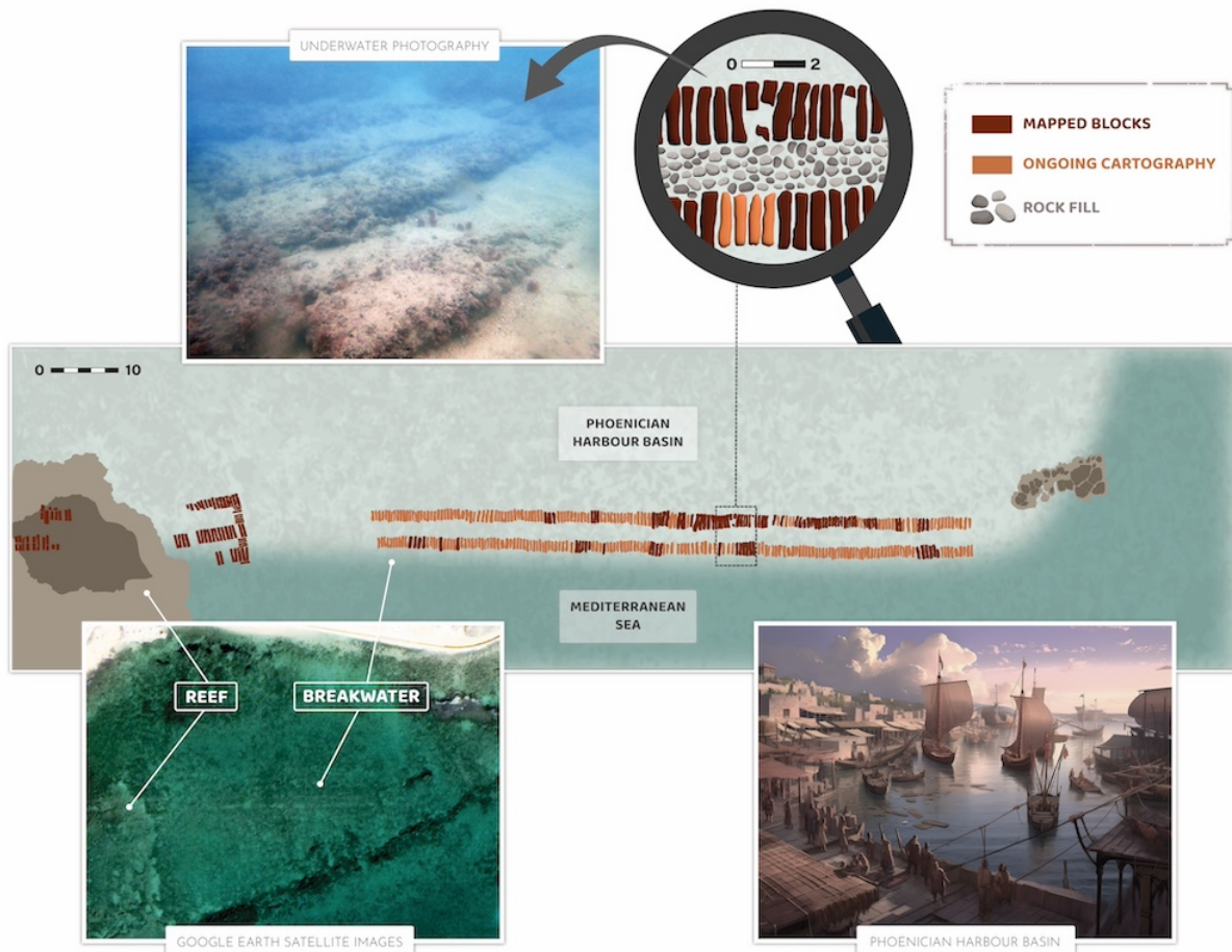
The east-west aligned, Phoenician-style breakwater discovered in 2019 extends over some 130 m. It displays a double alignment of oblong blocks (Figure by Sylvia Vinai, adapted from Goiran et al., 2021).
