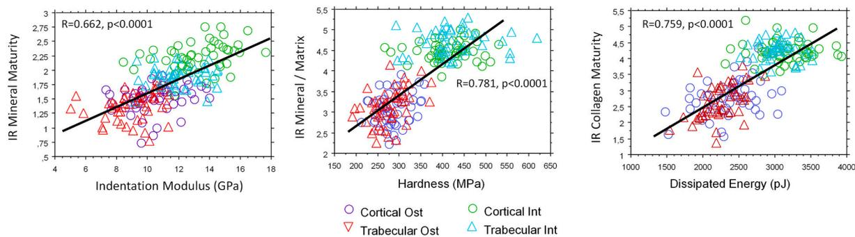
**Fig. 5.** Correlations between the nanomechanical and intrinsic variables in the 4 compartments. Each point is the mean of 10 and 5 BSUs for FTIRM and nano-indentation, respectively (n = 50 bone biopsies).
