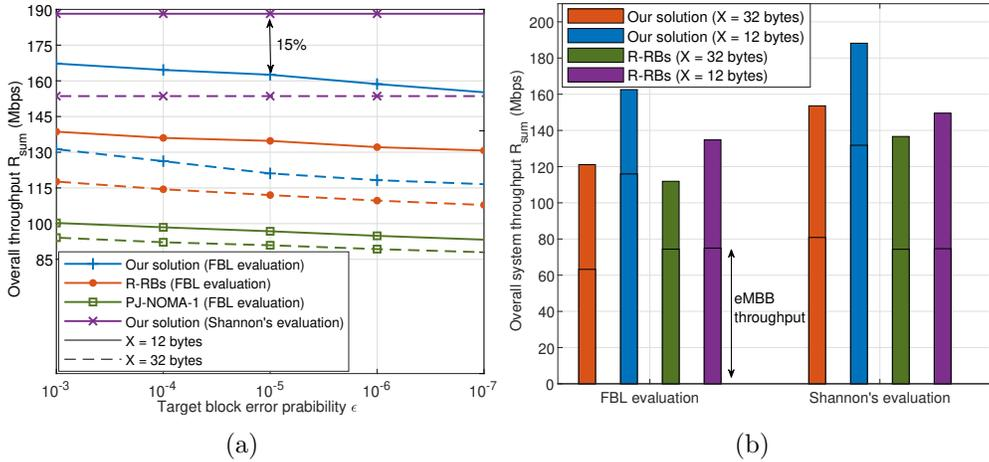
Figure 10: Performance comparison in terms of the overall system throughput (a) and the overall system throughput and eMBB sum-throughput ( $\epsilon = 10^{-5}$ ) (b). Different URLLC target block error probability and packet sizes are considered.
