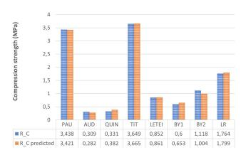
Figure 4: Comparison between actual measurements of R C and predictions.
