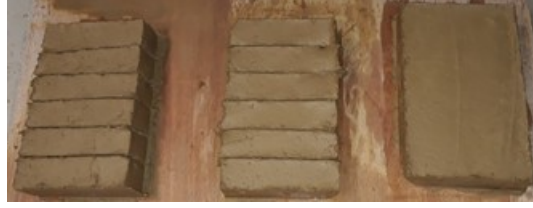
Figure 4: Preparation (a) and cutting of the fresh slabs to obtain six specimens (b)
