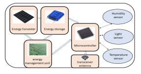
Fig. 2. Framework of an autonomous sensor node
