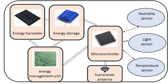
Fig. 2. Framework of an autonomous sensor node
