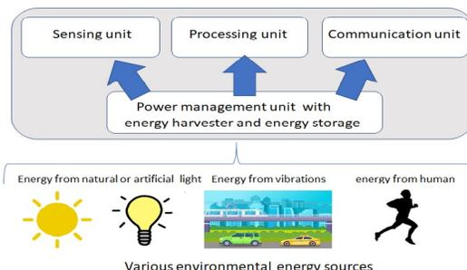
Fig. 1. Energy harvesting to supply small devices
