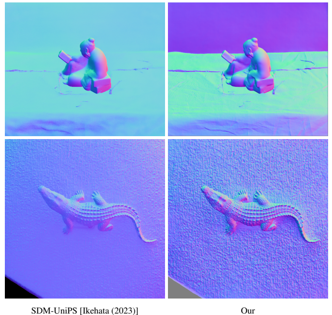
Fig. 11: Comparison on the Alligator object of SDM-UniPS [Ikehata (2023)] and the Reading object of DiLiGenT [Shi et al. (2016)] without masking background. We can see that considering the background does not degrade reconstruction of normals, and that we reconstruct more accurate details than SDM-UniPS [Ikehata (2023)].
