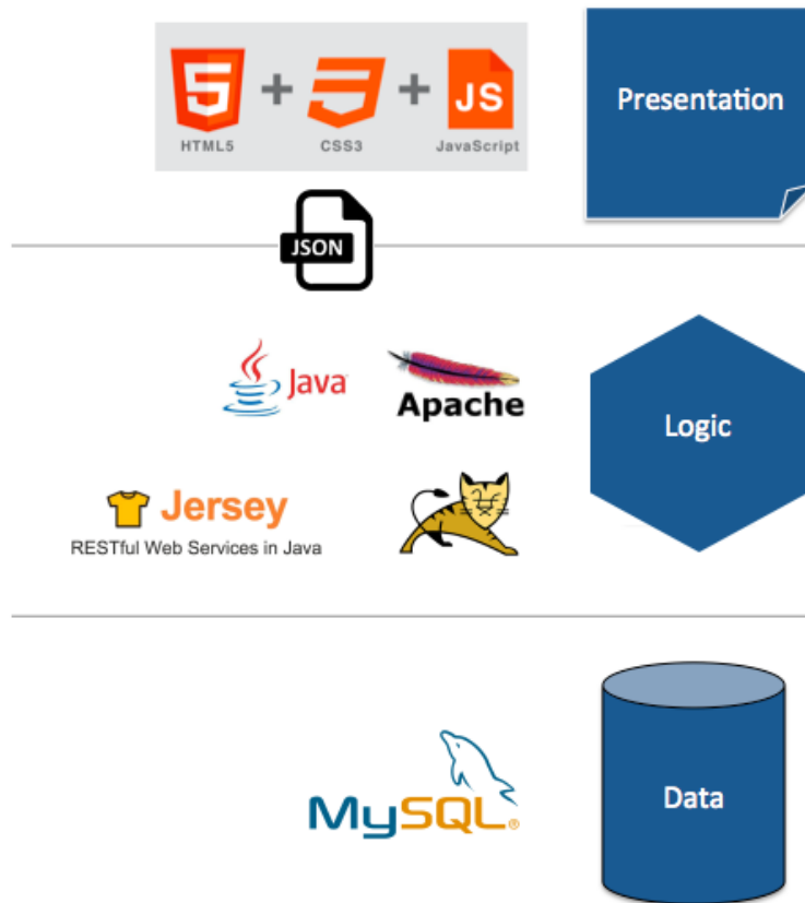
Figure 9: Web dashboard software stack
