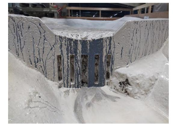
Slits of the open check dam clogged by gravels
