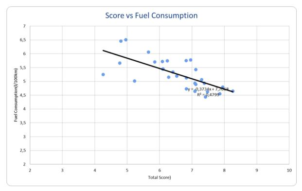
Figure 15: Okan University model, linking score with fuel consumption<sup>8</sup>
