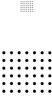
Fig. 2. Symmetrical Circle Grid with Two Rigidly Linked Pattern
