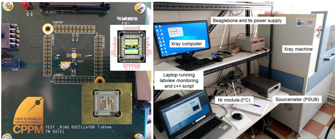
63 Figure 2. Left: DUT board with the chip bonded. Right: irradiation tests set-up.
