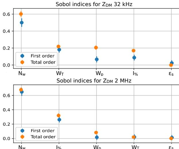
Fig. 6. Sobol indices for DM impedances at 32 kHz and 2 MHz
