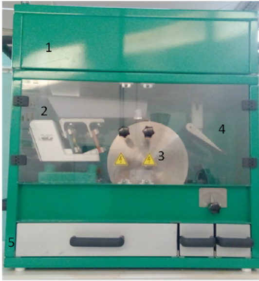
Fig. 3. Photography of the tribo-electrostatic roll-type separator : 1. Tribo-charging device; 2. Vibratory electromagnetic feeder; 3. Grounded electrode; 4. High-voltage electrode; 5. Three-compartment collector.
