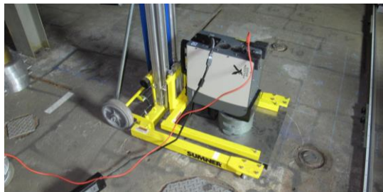
Fig. 3. Measurement setup # 1 with the HPGe detector for contamination measurement.
