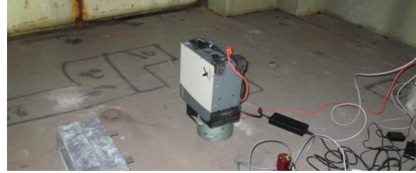
Fig. 4. Setup # 2 of the HPGe detector for background measurement.
