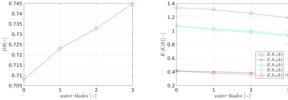
Figure 10: Dominance ratio (left) and  $k$ -eigenvalue separations (right) for EOLE water blade configurations. The first five order of eigenvalue separations are shown, in order, as:  $E.S._1(k)$  red circles,  $E.S._2(k)$  blue crosses,  $E.S._3(k)$  green squares,  $E.S._4(k)$  cyan diamonds and  $E.S._5(k)$  magenta triangles.
