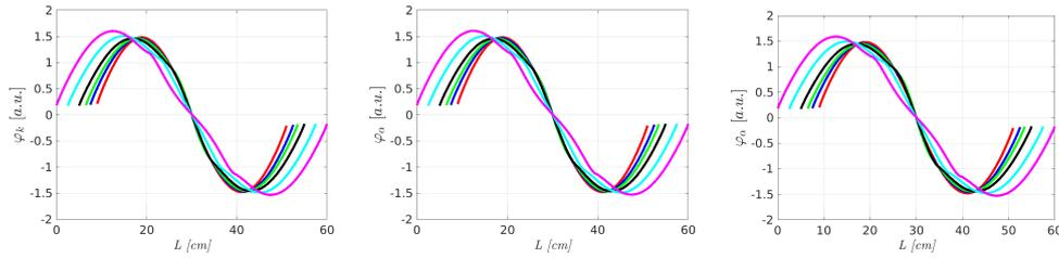
Figure 8: Spatial distribution of the  $k$  (left),  $\alpha$  (center) and prompt  $\alpha$  first-order eigenmodes for the 1D heterogeneous as a function of the size  $L$  of the system. Color legend according to the ascending order of the size  $L$  of the system is:  $L = 42$  cm red,  $L = 45$  cm blue,  $L = 47$  cm green,  $L = 50$  cm black,  $L = 55$  cm cyan and  $L = 60$  cm magenta.
