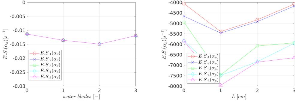
Figure 11: Delayed (left) and prompt (right)  $\alpha$ -eigenvalue separations for EOLE water blade configurations. The first five order of eigenvalue separations are shown, in order, as:  $E.S.1(\alpha)$  red circles,  $E.S.2(\alpha)$  blue crosses,  $E.S.3(\alpha)$  green squares,  $E.S.4(\alpha)$  cyan diamonds and  $E.S.5(\alpha)$  magenta triangles.
