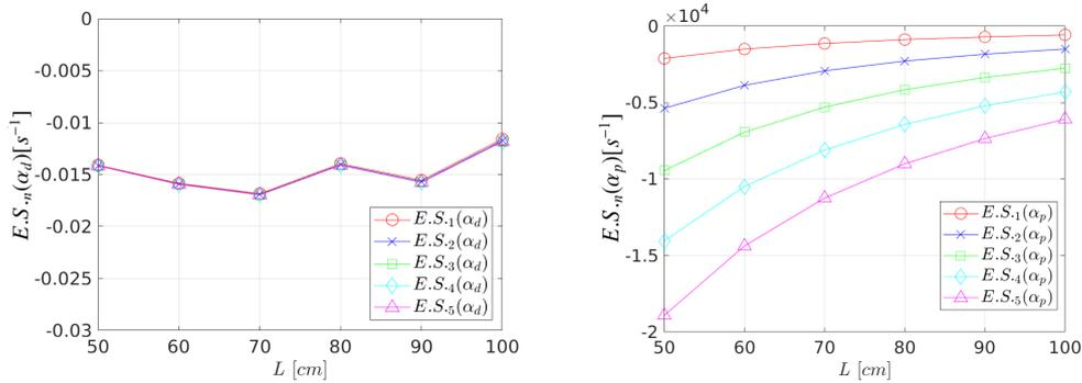
Figure 4: Delayed (left) and prompt (right)  $\alpha$ -eigenvalue separations for the 1D homogeneous configuration with leakage boundary conditions as a function of the size  $L$  of the system. The first five order of eigenvalue separations are shown, in order, as:  $E.S._1(\alpha)$  red circles,  $E.S._2(\alpha)$  blue crosses,  $E.S._3(\alpha)$  green squares,  $E.S._4(\alpha)$  cyan diamonds and  $E.S._5(\alpha)$  magenta triangles.
