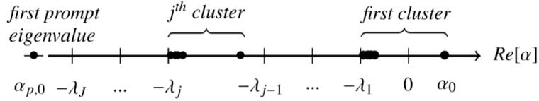
Figure 1: Typical spectrum of  $\alpha$ -eigenvalues for a super-critical system. Sketch inspired by the reference ([Sanchez and Tomatis, 2019](#)).
