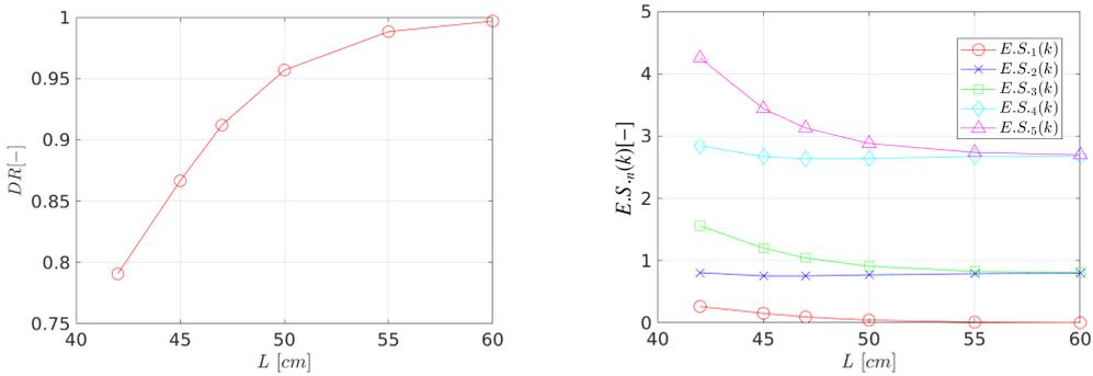
Figure 5: Dominance ratio (left) and  $k$ -eigenvalue separations (right) for the 1D heterogeneous configuration as a function of the size  $L$  of the system. The first five order of eigenvalue separations are shown, in order, as:  $E.S._1(k)$  red circles,  $E.S._2(k)$  blue crosses,  $E.S._3(k)$  green squares,  $E.S._4(k)$  cyan diamonds and  $E.S._5(k)$  magenta triangles.
