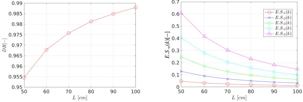
Figure 3: Dominance ratio (left) and  $k$ -eigenvalue separations (right) for the 1D homogeneous configuration with leakage boundary conditions as a function of the size  $L$  of the system. The first five order of eigenvalue separations are shown, in order, as:  $E.S._1(k)$  red circles,  $E.S._2(k)$  blue crosses,  $E.S._3(k)$  green squares,  $E.S._4(k)$  cyan diamonds and  $E.S._5(k)$  magenta triangles.
