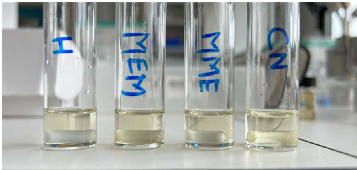
Figure S13 Pictures of the solutions obtained after addition of 2-cyclohexen-1-one (2 mL) to the H, MEM, MME, CN ILs (0.5 mL).
