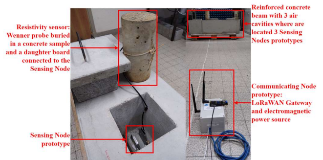
Fig. 6. Photographs of an experimental set-up composed of Sensing Nodes embedded in a reinforced concrete beam.
