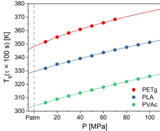
**Figure 4.** Glass transition temperature as a function of pressure for PETg in red, PLA in blue and PVAc in green. The lines correspond to the approximation of the experimental data with the Andersson's fit function.
