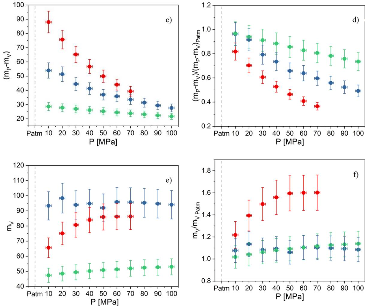
**Figure 9.** a) Activation volume  $\Delta V^\#$  at  $T_g(P)$  (the lines correspond to the one-phase exponential decay function), b)  $\Delta V^\#$  normalized to its value at  $P_{atm}$ , c) volumetric contribution  $(m_P - m_V)$ , d)  $(m_P - m_V)$  normalized to its value at  $P_{atm}$ , e) thermal contribution  $m_V$  and f)  $m_V$  normalized to its value at  $P_{atm}$  as the function of pressure for PETg in red, PLA in blue and PVAc in green.
