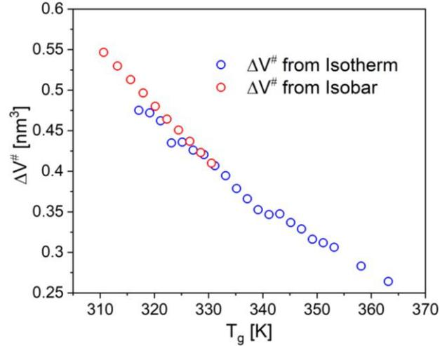
**Figure 6.** Activation volume  $\Delta V^\#$  at the glass transition temperature  $T_g$  calculated from isothermal measurements and **Equation (4)** in empty blue circle, and from isobaric measurements and **Equation (8)** in empty red circles for PVAc.
