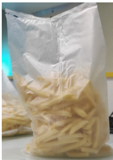
FIGURE 7 Hot sealed film of PHBV/PBSA/ATBC10/0.2Lp filled with 625 g of parfried frozen French fries. [Color figure can be viewed at wileyonlinelibrary.com ]
