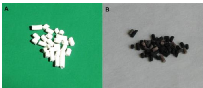
Figure 16: The surface of Na-ZSM-5 catalyst (A) before and (B) after the measurement of activity [105]
