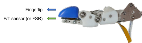
Fig. 14 Mounting of sensors on the fingertip.
