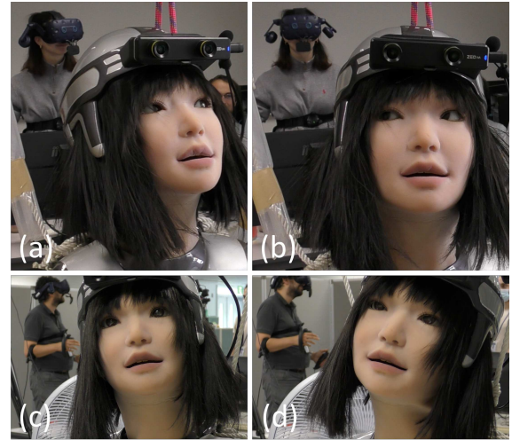
Fig. 22 Neck motion: looking left-right using the yaw joint in (a) and (a), and head tilting using the roll joint in (c) and (d).
