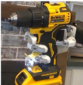
Fig. 13 Power grasping (heavy wrap while operating drill)
