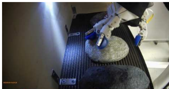
Fig. 35 Screenshot taken during the execution of the rocks task, specifically when rubbing the second rock (smoothest). Note that the operator did not have a visual of the rocks; he just knew their approximate position inside the box.
