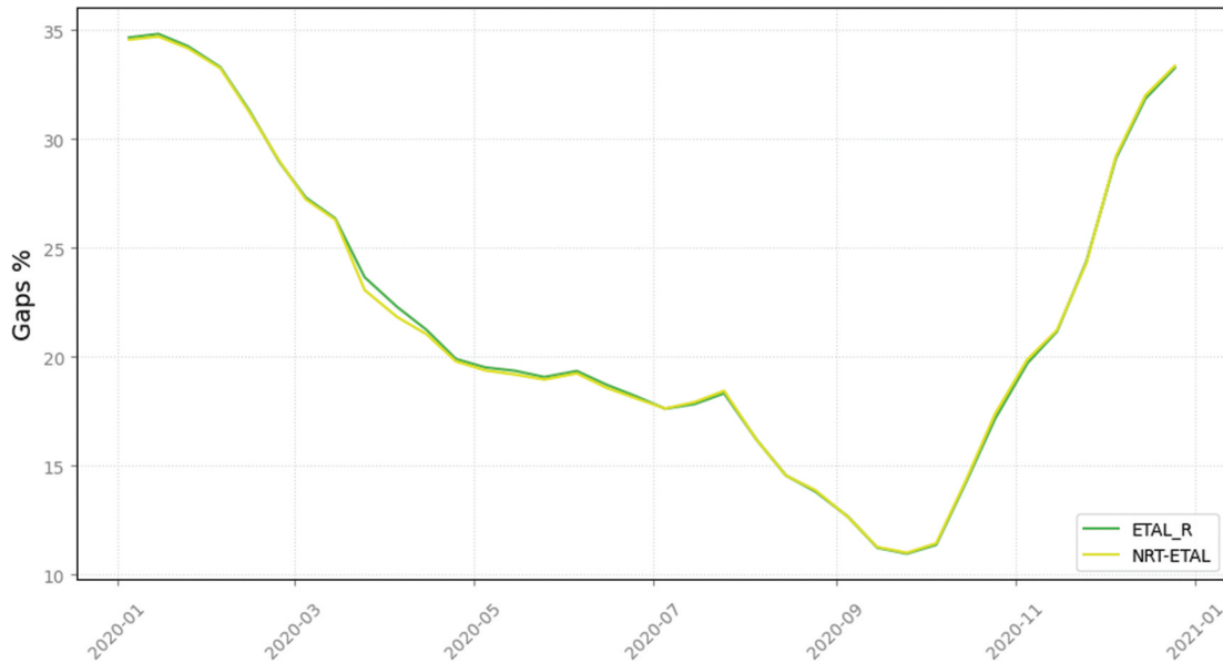
Figure 10. Percentage of missing data for ETAL-R and NRT ETAL AL-BB-BH averaged over the globe for 2020.
