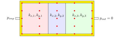
Figure 7: System representing the "reality". The zones with different permeabilities are illustrated with different colors and separated by lines.
