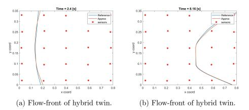
Figure 12: Comparison between the flow-front prediction when using the Gappy POD and the simulated experience for two different time instants.
