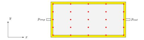
Figure 2: 2D mold with  $n_{s,x} = n_{s,y} = 5$  sensors represented by red dots; the yellow color represents the race-track zone.
