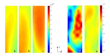
Figure 1: a, b and c: Longitudinal strain fields measured by DIC at three different times at static condition for zero strain, d: Longitudinal strain field measured by DIC at  $600\hat{A}^{\circ}C$  during a tensile test, e: Same longitudinal strain field after a correction with the Gaussian low pass filter (radius r=5, sigma=2)
