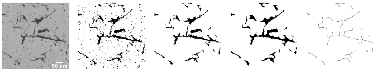
Fig. 2. Illustrations of the four processing operations used to transform a raw image of the reference ceramics obtained by optical microscopy into a skeletonized image of their inter-granules porosity. From left to right: initial image, thresholding, elimination of unwanted objects based on the circularity of connected components in the binary image, smoothing of the edges of the pores by a morphological closing of appropriate size and skeletonization of the resulting objects.
