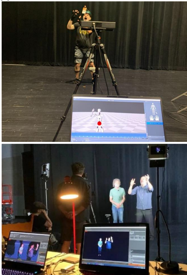
Figure 1. Top: Performance-capture of Peter Cook including body and face. Bottom: Depth video capture of the performance of Peter Cook and Kenny Lerner in the studio.
