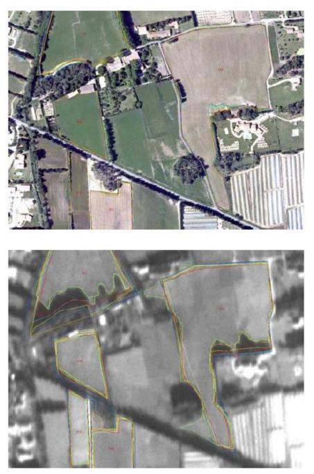
Figure 3. Example of area measurement on orthophoto and Cartosat1 images
