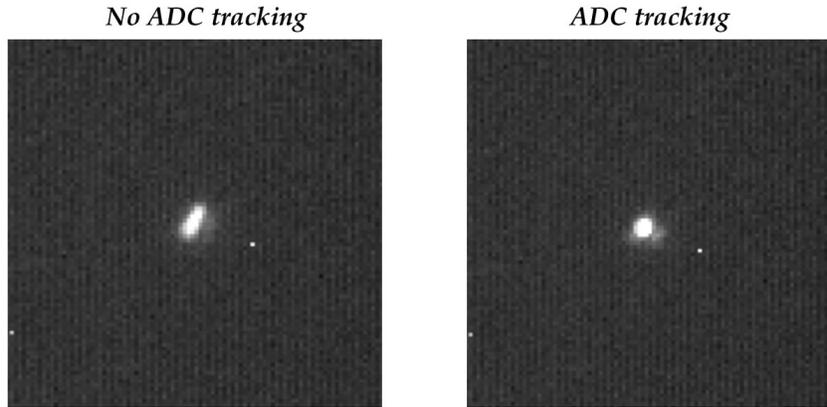
Figure 8: the ADC tracking test; after some refinement, we could achieve a PSF residual ellipticity  $< 1.1$  at an elevation of  $45^\circ$  and considering the full wavelength range (from Y to H band) of SHARK-NIR
