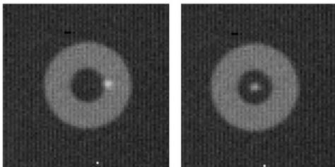
Automatic **pupil alignment** procedure tested on sky and working in maximum 3-4 iterations. Telescope pupil and instrument pupil mask co-aligned with an accuracy < 50 mas, within the requirements.
