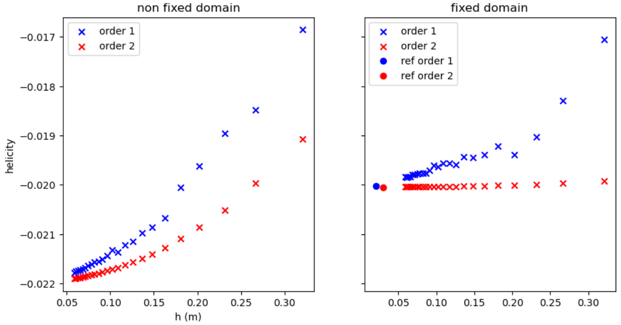
Figure 3: On the left, we provide better and better approximations of the surface to the mesher. We then plot the characteristic size of an element versus the harmonic helicity. On the right, we mesh with different characteristic size h the same polyhedral approximation of the continuous surface.
