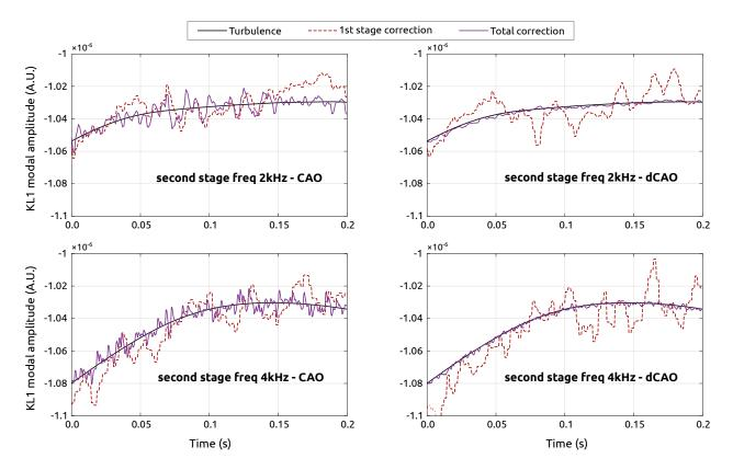
Figure 4. Temporal trajectories of first mode from the KL basis of the HODM in presence of turbulence (black), 1<sup>st</sup> stage correction (dashed red) and total correction (purple) for 2 frequency configurations (2 kHz and 4 kHz for SAXO+, the 1<sup>st</sup> stage running at 1 kHz), for CAO (left) and dCAO (right).
