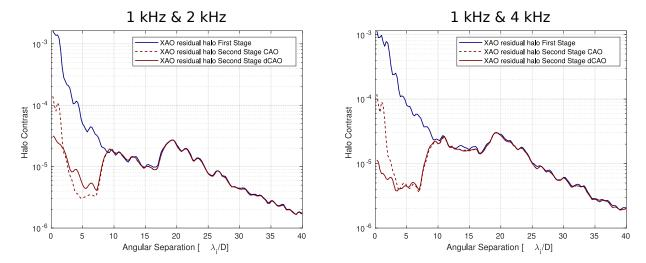
Figure 3. Residual halo contrast curves estimated in closed-loop for both frequencies configurations and with CAO (red dashed line) and dCAO (red plain line). The contrast obtained with the 1<sup>st</sup> stage only is also displayed (blue plain line).
