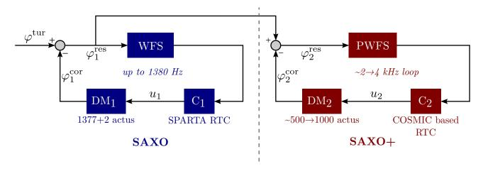
Figure 1. Two-stage CAO setup for SPHERE+, showing dimensional features of the existing system (SAXO) and of the foreseen  $2^{nd}$  stage (SAXO+).
