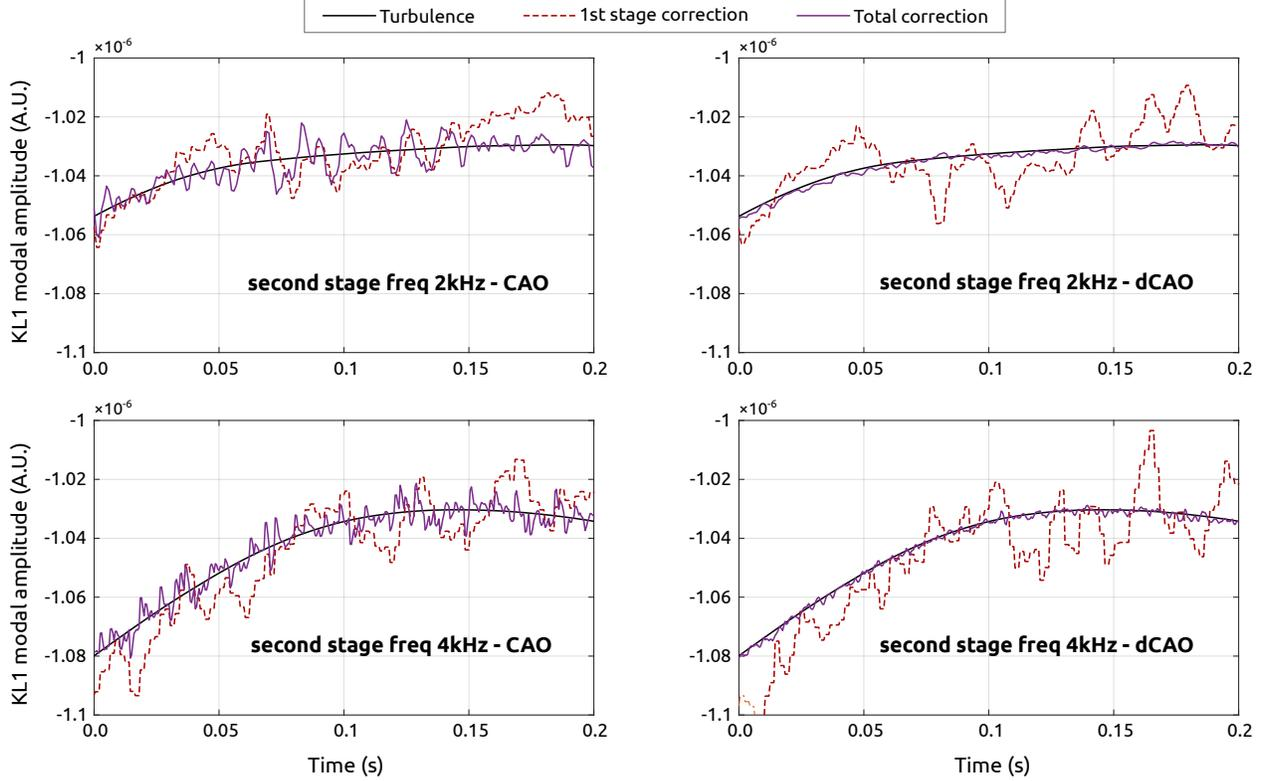
Figure 4. Temporal trajectories of first mode from the KL basis of the HODM in presence of turbulence (black), 1<sup>st</sup> stage correction (dashed red) and total correction (purple) for 2 frequency configurations (2 kHz and 4 kHz for SAXO+, the 1<sup>st</sup> stage running at 1 kHz), for CAO (left) and dCAO (right).
