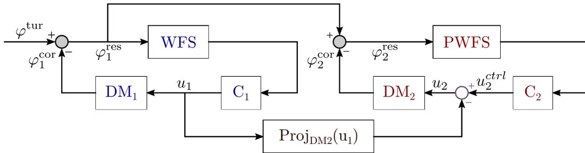
Figure 2. Block diagram of a dCAO setup. The commands from the 1<sup>st</sup> stage are projected onto the 2<sup>nd</sup> stage DM basis (it can be either zonal or modal) and subtracted from the commands calculated by the 2<sup>nd</sup> stage controller.
