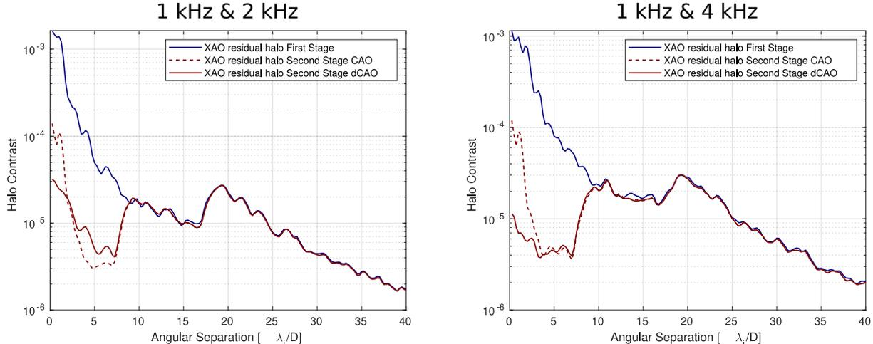
Figure 3. Residual halo contrast curves estimated in closed-loop for both frequencies configurations and with CAO (red dashed line) and dCAO (red plain line). The contrast obtained with the 1<sup>st</sup> stage only is also displayed (blue plain line).
