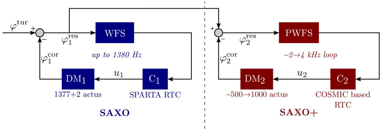
Figure 1. Two-stage CAO setup for SPHERE+, showing dimensional features of the existing system (SAXO) and of the foreseen 2<sup>nd</sup> stage (SAXO+).
