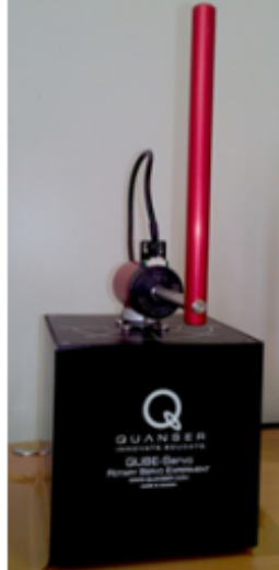
Figure 6: The Furuta pendulum system.
