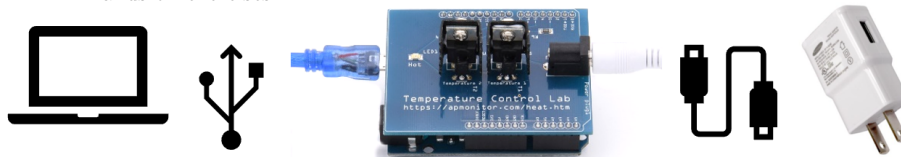
Figure 4: The Temperature Control Lab (TCLab) connects to a computer for Python or MATLAB hands-on exercises.
