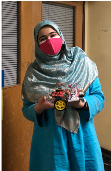
Figure 1: A proud student showing off her final project, the voice-controlled robot car in EECS16B at UC Berkeley at the end of her first year. The project uses principal-components-analysis to learn the voice commands and pole-placement for control of the car.
