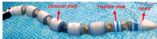
Fig. 1. First swimming test of Natrix on the water surface.
